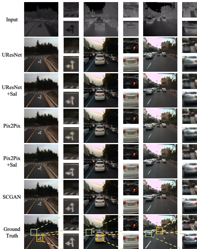
Fig. 9. Comparison of multispectral image colorization results between the proposed SCGAN and other approaches [2], [36]. The first row is the multispectral input while last row is ground truth visible RGB images. Row 2-6 represent colorization results of proposed SCGAN and other methods. We highlight two patches in each pair and the location is indicated by green and yellow rectangles.
