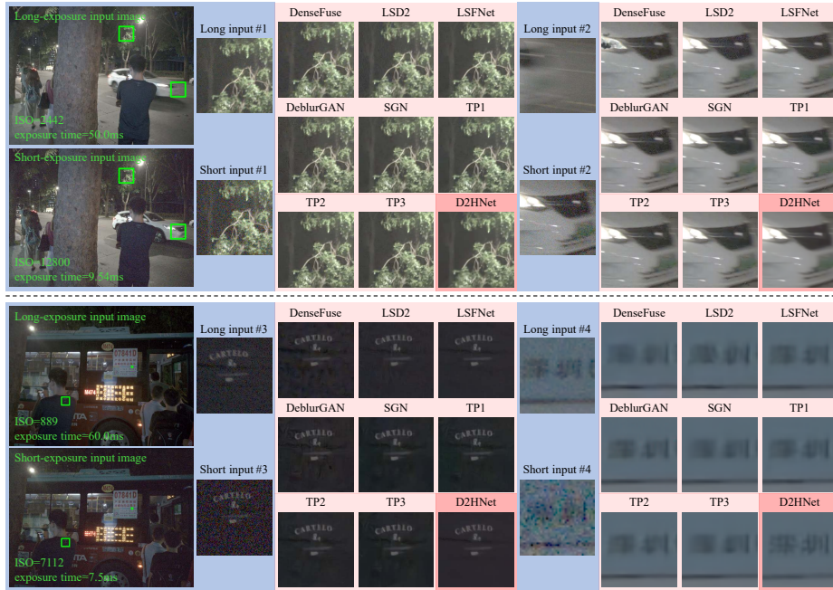
Fig. 6. Visual comparisons of the proposed D2HNet with other methods. More results on both real photos and validation images are in the supplementary material.
